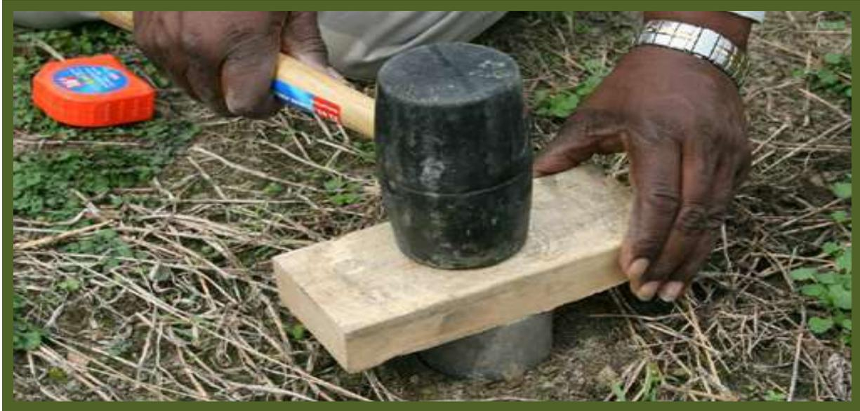
Figure 2. Seating the bulk density sampling ring into the soil to get a representative soil sample. The wood board and mallet are used to get a full bulk density sample.
