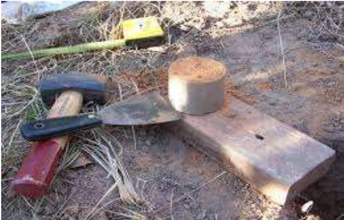
Figure 3. A full, trimmed bulk density sample which is ready to be placed in the gallon ziplock sampling bag as one of the four composite bulk density samples.
