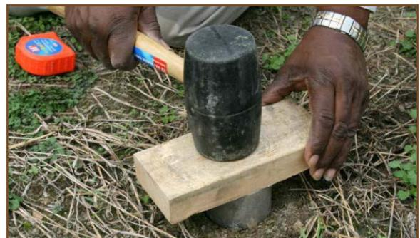
**Figure 6. Drive ring to 3-inch depth.**
