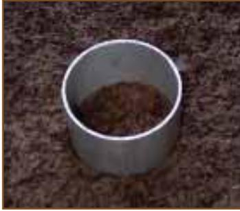
**Figure 7. Ring driven to 3-inch depth.**
